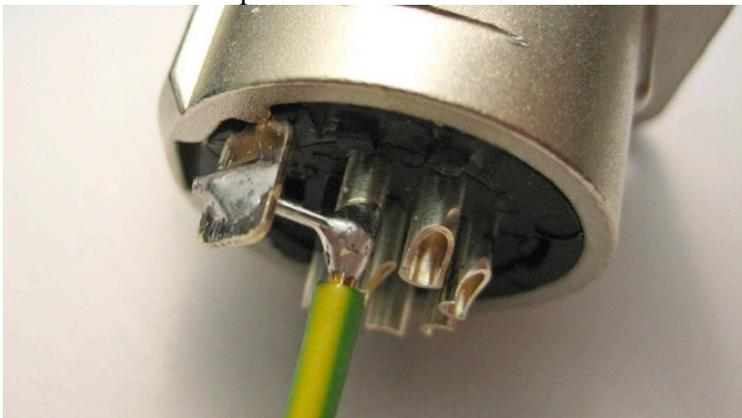
5. If you have some small diameter heat shrink, you can cut 6 pieces approximately 3/8" (9.5mm) long and slip them onto the remaining wires. The heat shrink is not supplied and not 100% necessary. If you do clean work with your wires and soldering, you will have no issues.
