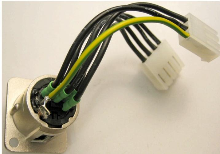
8. Insert the power cable assembly into the DC In hole of the 511-Back panel and secure with the supplied hardware. Set the 511-Back panel to the side until later.
