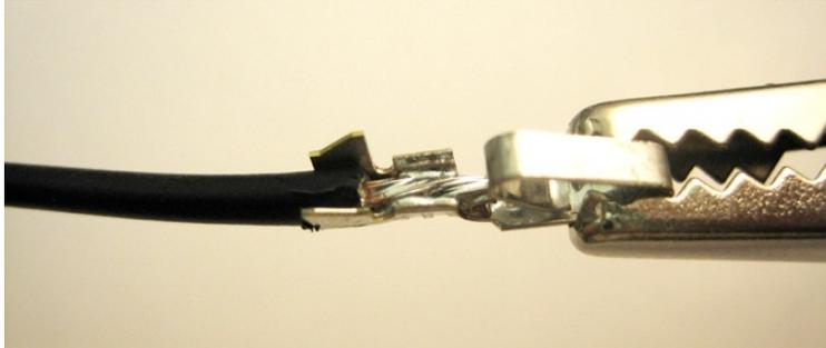
3. Crimp the tabs closed with a needle nose pliers. This must be done or the terminals will not slide into the receptacle housing properly.
