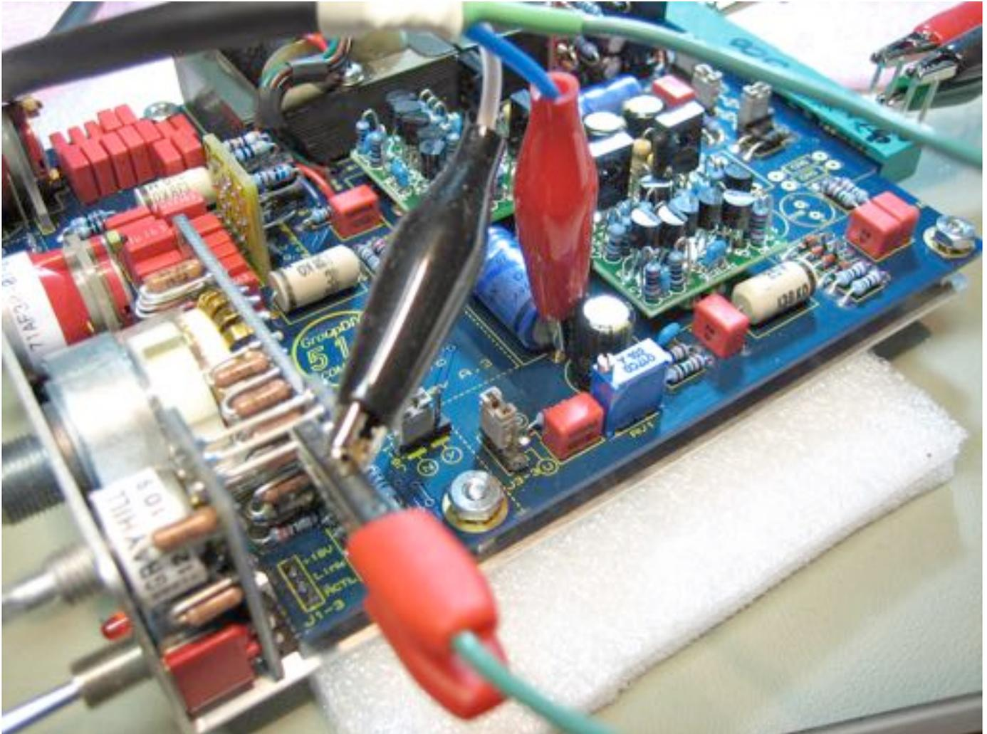
Alterations may need to be made if the inputs of your DAW do not like pin 3 shorted to ground. Some may need to let that float. If you are using a DMM or a scope, these are the same points where you can hook your probes.
